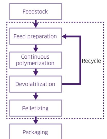
Polystyrene block flow diagram
