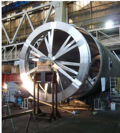
Manufacturing of Disc Ring Autoclave
